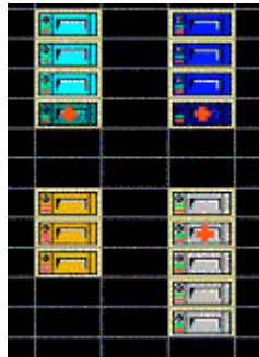
Figure 4- 33: Identifying Failed Drives
