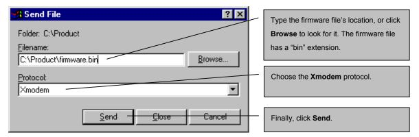
Figure 3-10 Example Xmodem Upload
