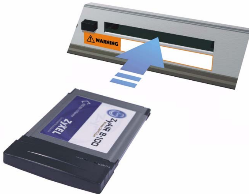
Figure 411 WLAN Card Installation
